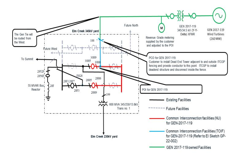
Figure 1 GEN 2017-119 Interconnection Substation One Line
